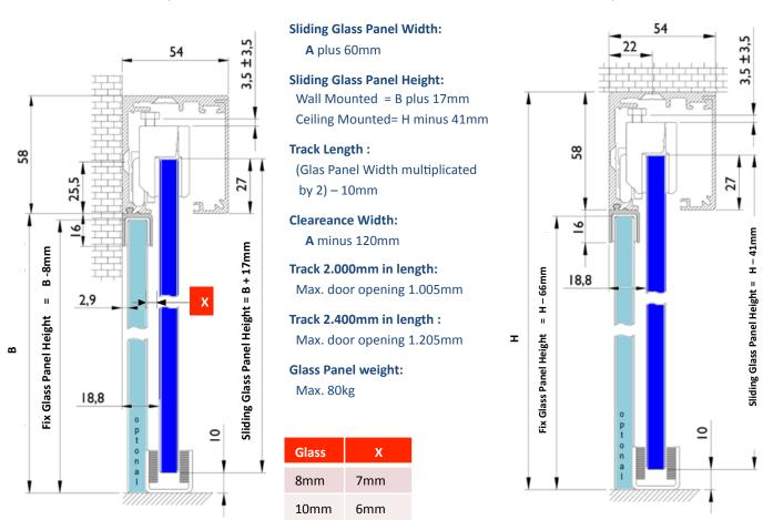
Please note: This is a recommandation, you have the possibility to change some of this recommendation, if needed and possible. Min. width of sliding glass panel is 750mm in combination with the Soft Close Kit. Min. track length is 960mm.
